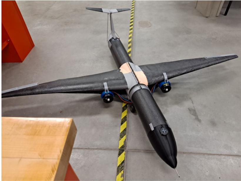
**Figure 1.2:** First iteration of the Truss-Braced Wing
