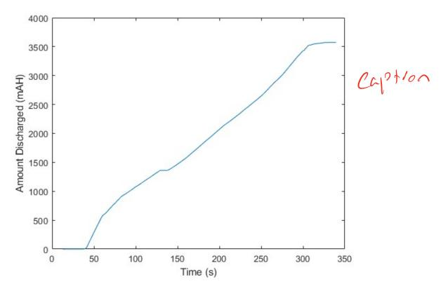
This graph shows the total lost milliamp-hours(mAH) vs. time since battery connection. This is primarily useful when further processing is completed. Although, the battery did end with 3572 mAH depleted from the 5000 mAH rated battery.
