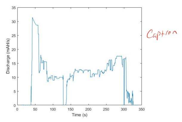
This is a graph of milliamp-hours per second(mAH/s) battery connection. This was accomplished by using the backward difference approximation for the instantaneous derivative. For this flight, the mea-
