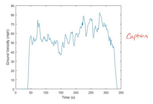
This graph shows the flight speed as a function of time since battery connection, measured by the onboard GPS module. There is no airspeed data for this flight. Thus ground speed is the only metric available to discuss. The flight reached a maximum of 82mph and a minimum of 36mph. From system time of 45 seconds to 325 seconds, the flight averaged a speed of 58mph.
